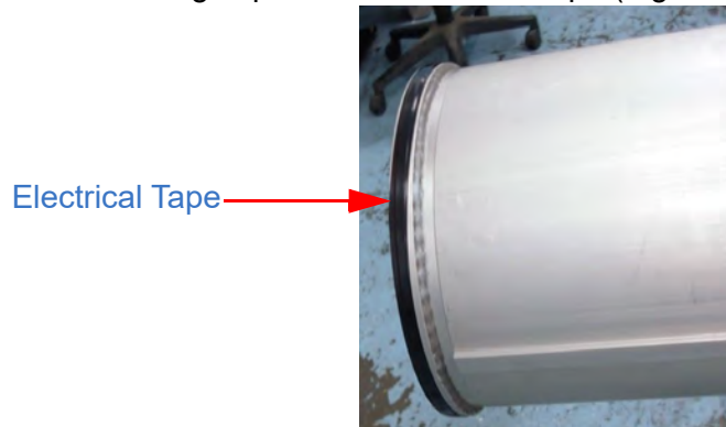
Figure 8-15 Electrical Tape Securing Wear Ring
